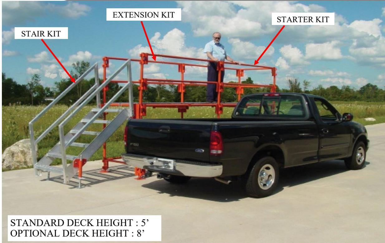
Perimeter Security Products is constantly striving to design products that will make the work environment a safer and efficient place. We recognized the need to streamline and improve vehicle inspections and as a result we have designed the Vehicle Inspection Platform (VIP). Currently at most gate entrance; guards are required to visually inspect truck beds and trailers before allowing entry. The VIP can be used at border crossings or for rail car inspections.
