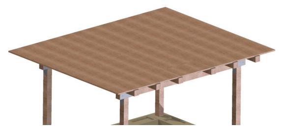
Stretch the rubber roof material over the top, pulling it down and fasten it on the underside of the roof panels. Using a sharp knife slit the material at the side seams of the access panel allowing it to be raised up.
