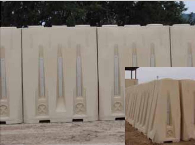
The **Houston Barricade** is 8' tall by 4' wide. It provides blast protection using sand for mitigation. No heavy equipment is necessary to install the barricade. Forklift pockets make it possible to easily reposition sections as threats change. The Houston Barricade is made of high density polyethylene. In demonstrations this barricade has shown it's ability to catch shrapnel and eliminate rebounds and ricochet.
