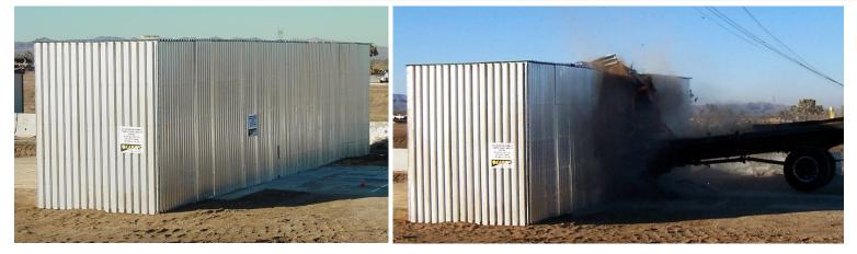
The Revetment Wall was specifically designed to protect critical infrastructures, military personnel and innocent civilians from terrorist attacks involving vehicles with explosive weapons. The 10' tall x 8' wide x 40' long Revetment Wall has been certified to stop a 15,000 lbs. vehicle traveling at 50 mph (Department of State K12 certification and ASTM F2656-07 / M50 Certification).
