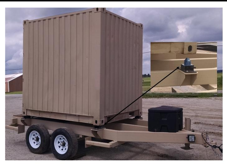
The Container Trailer can be used to transport Quadcon (5 x 8 ft.) Containers or Tricon (6.5 x 8 ft.) Containers. The containers are loaded onto the locking lugs by forklift or other material handling equipment. Once loaded onto the trailer, it can be quickly locked into place for transportation.
