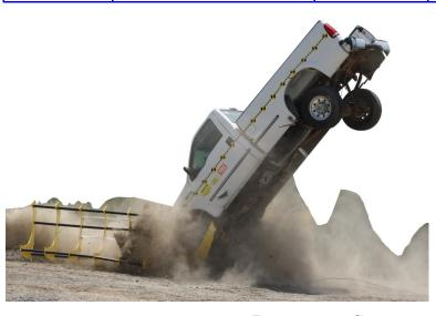
On May 15, 2010, Perimeter Security Products performed a crash test on the Raptor Vehicle Barrier. The testing was based on ASTM Vehicle Crash Test Standard (ASTM F265-07). A 3/4 Ton Pickup Truck weighing 5,200 lbs. was crashed into the Raptor Vehicle Barrier (free standing set on top of crushed rock) at 40 MPH.
