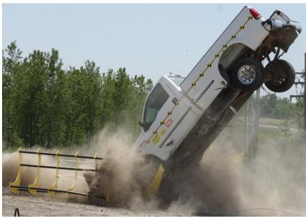
On May 15, 2010, Perimeter Security Products performed a crash test on the Raptor Vehicle Barrier. The testing was based on the ASTM Vehicle Crash Test Standard (ASTM F265-07). A 3/4 top pickup truck weighing 5200 lbs was crashed into the Raptor Vehicle Barrier (free standing on crushed rock) at 40 mph.
