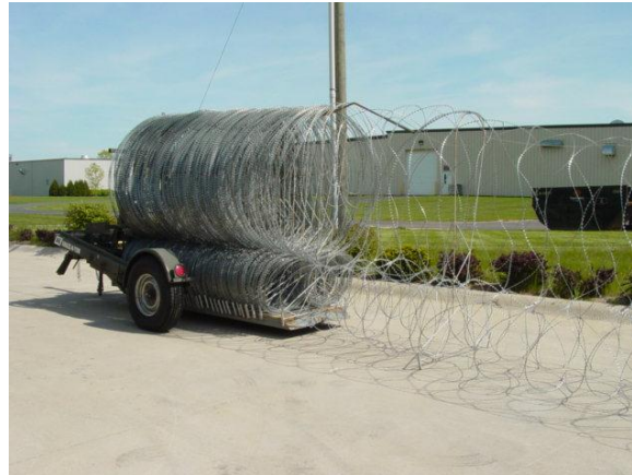
Figure 2: Wire Barrier System being deployed
